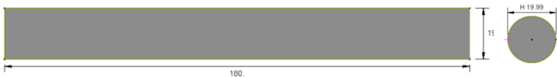
Fig. 3.22: Dimensions of S235*(1) material tensile test specimen (DISSIPABLE, 2021).
