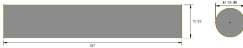
Fig. 3.23: Dimensions of S235*(2) material tensile test specimen (DISSIPABLE, 2021).
