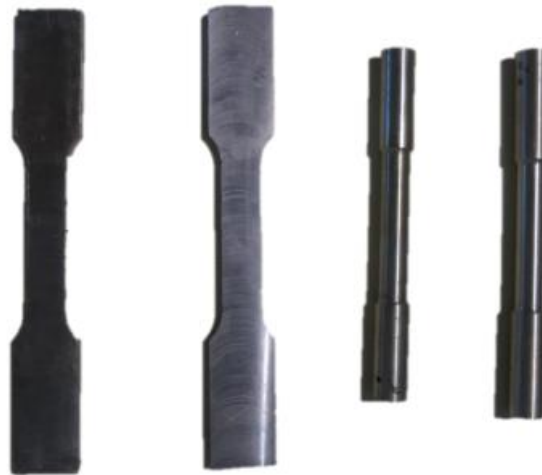
Fig. 3.16: Tensile test specimens of S355, HSS, StS and S235 materials, respectively (DISSIPABLE, 2021).
